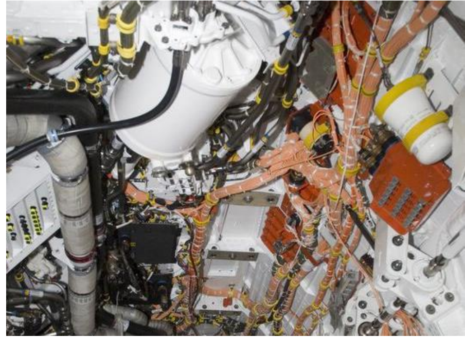
JSF wiring (28km wiring, 20k connectors)!
