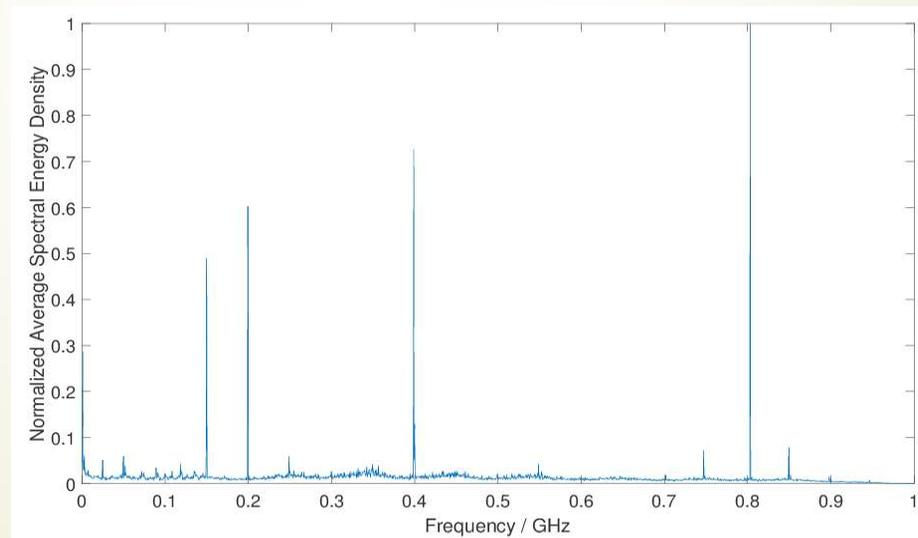
The normalized average spectral energy density at 3 mm height from the *Intel Galileo board*
