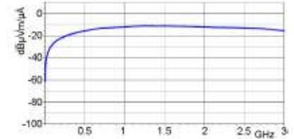
(b) Frequency characteristic of RF probe used in measurements.
