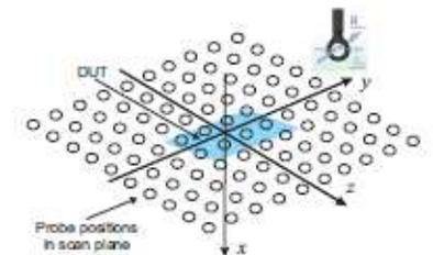
Fig. 3. Near-field probe positions.
