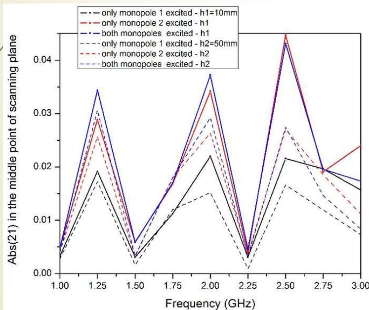
Transfer function describing the coupling between monopoles and RF loop probe placed at the point in the middle of scanning plane above the enclosure lid with one square aperture
