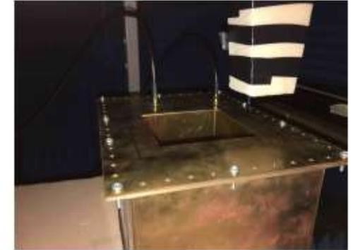
(c) Experimental enclosure with RF loop probe placed above the removable enclosure lid.
