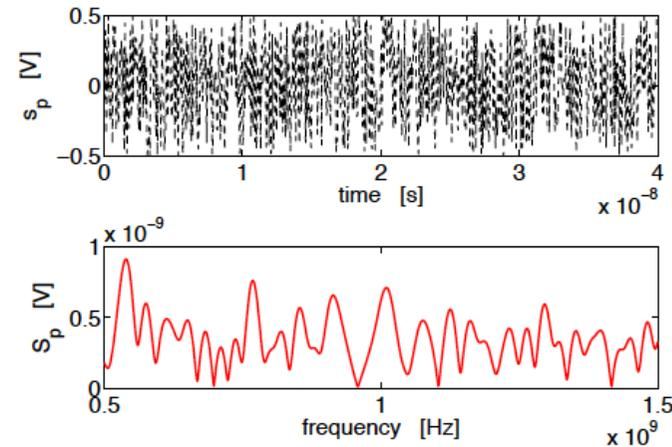
Random (uniformly distributed) voltages driving cable wires
